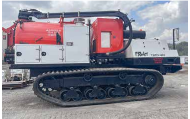
Aggressive Power Sweeping expands their scope to include a tracked vehicle that can be used as a Vacuum Truck, Drill Rig, Water Truck, Pipe Rack, or End Dump by swapping out the back of the equipment.
