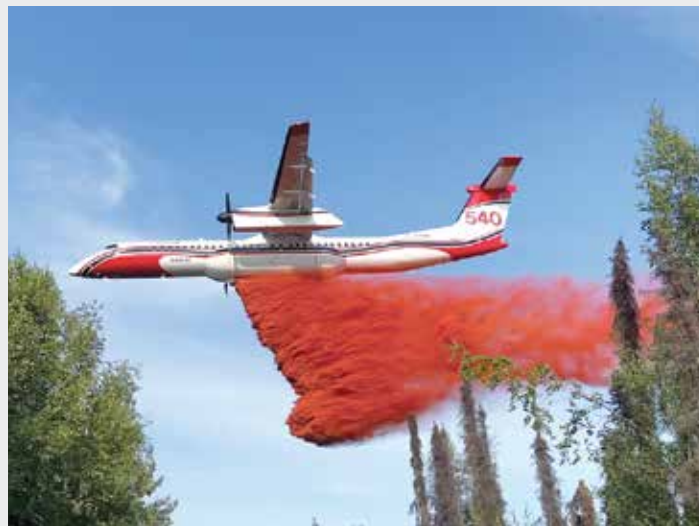
Conair's Dash 8-Q400AT Tanker 540 dropping retardant in Alaska. Conair coordinated with local fire departments to construct direct firelines.
