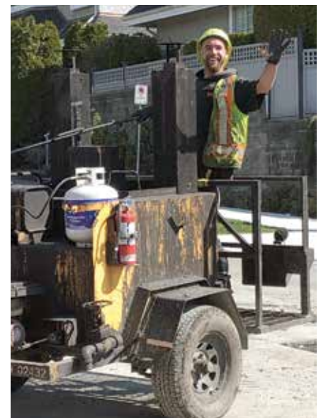
Sean Stewart running spray pot for an overlay in North Vancouver with BA Blacktop
