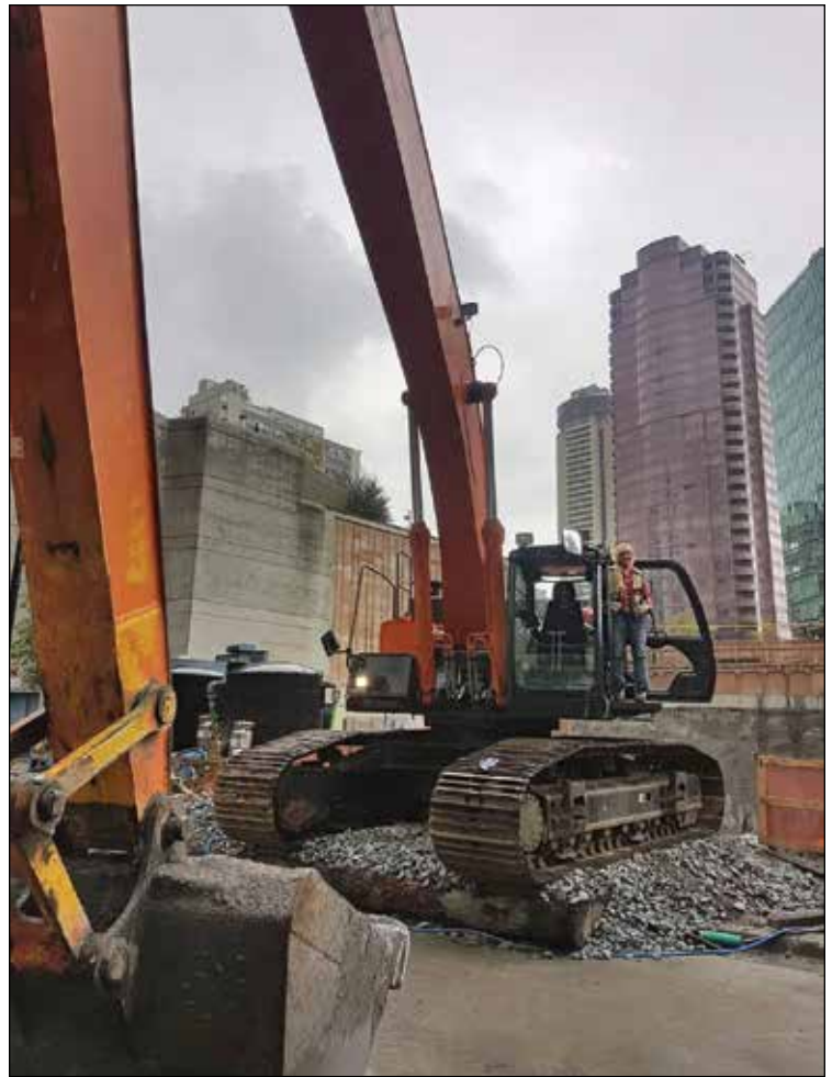
Emily Jansson running a 470 long stick Hitachi crane, working for Mainland Group of Companies. The crane is sitting on the edge of 90 foot excavation at Cardero St & W Georgia St in Vancouver.
