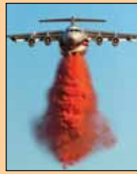
Conair's jet powered Avro RJ85, a variant of a British Aerospace BAe-146. The RJ85 has been converted into a Type 3,000-gallon air tanker. —Photo courtesy of Conair
