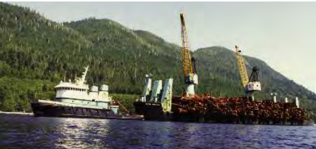
The log barge Rivtow Hercules towed by the ocean-going tug Captain Bob loads logs off the water along B.C.'s rugged coastline. Operating engineers have been manning log barges for 50 years.
