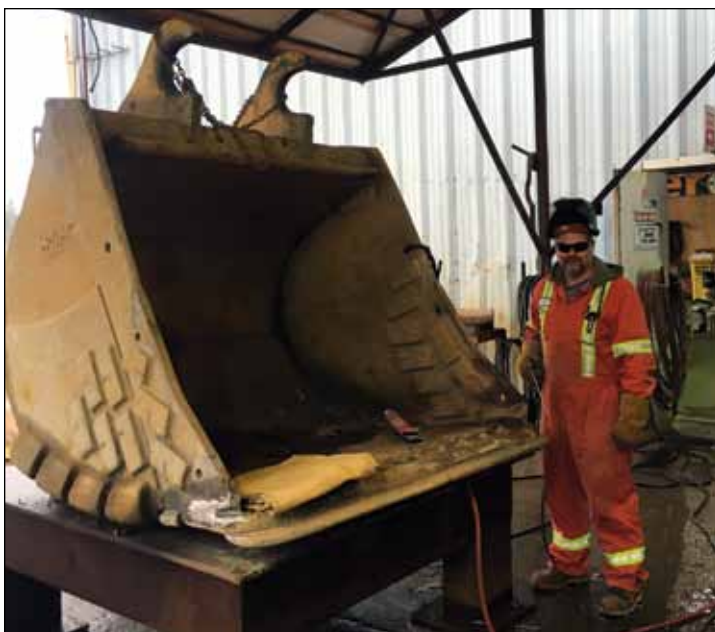
Brother Eric Miller working at Pitt River Quarry, doing maintenance welding on a Cat 349 excavator clean-up bucket. Photo: Brother Frank Carr
